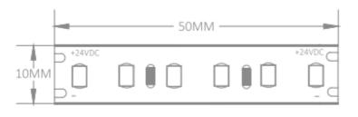
V-XXXX m, 11w/m, 16w/m, 23w/m 8x100mm, 10x50mm, 10x50mm, 10x25mm nm, 8LEDs 100mm, 6LEDs 50mm, 6LEDs 25mm
